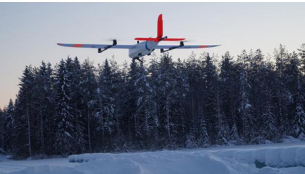
Drone equipped with electromagnetic survey system for mineral exploration
