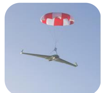
Figure 13: UAV outfitted with a parachute as a further safety measure
